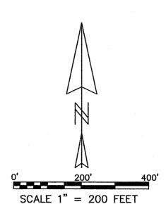
BASIS OF BEARING: BEARING BETWEEN MONUMENTS FOUND AT THE SOUTHWEST SECTION CORNER AND THE SOUTH QUARTER CORNER. OCRS NORTH CENTRAL ZONE. NAD 83 (2011) EPOCH 2010.00 CS 7652 CITES THIS BEARING AS NORTH 89'40'31" EAST AS SHOWN.
