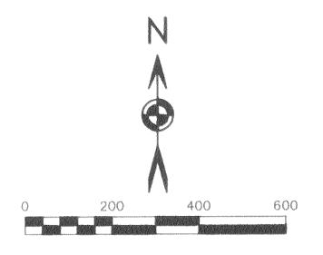
BASIS OF BEARINGS: N 86'59'52" E ALONG THE NORTH LINE OF THE N.E. QUARTER OF SECTION 24 BETWEEN MONUMENTS FOUND AS NOTED PER CS 2007108.
