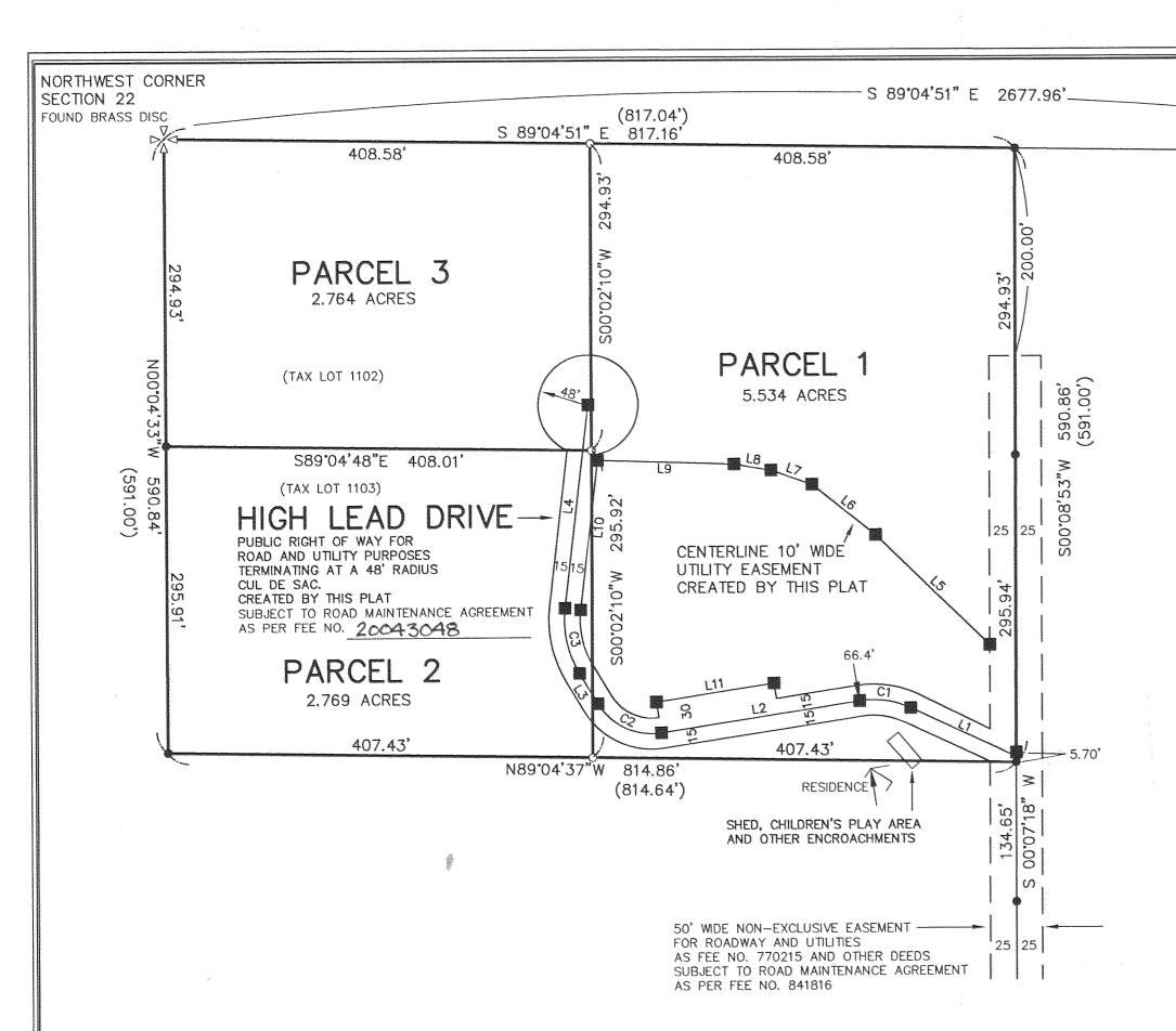
LINE TABLE **BEARING** LENGTH LINE 111.46 S64°52'50"E 193.54 N81'04'48"E 34.06 N30°52'43"W N06'39'37"E S45'38'45"E 152.69 78.22 S51°34'39"E 41.82 S70°45'52"E 36.05 S80'27'22"E 131.32 S88°04'12"E L10 N06°39'37"E 114.66 N81°04'48"E
