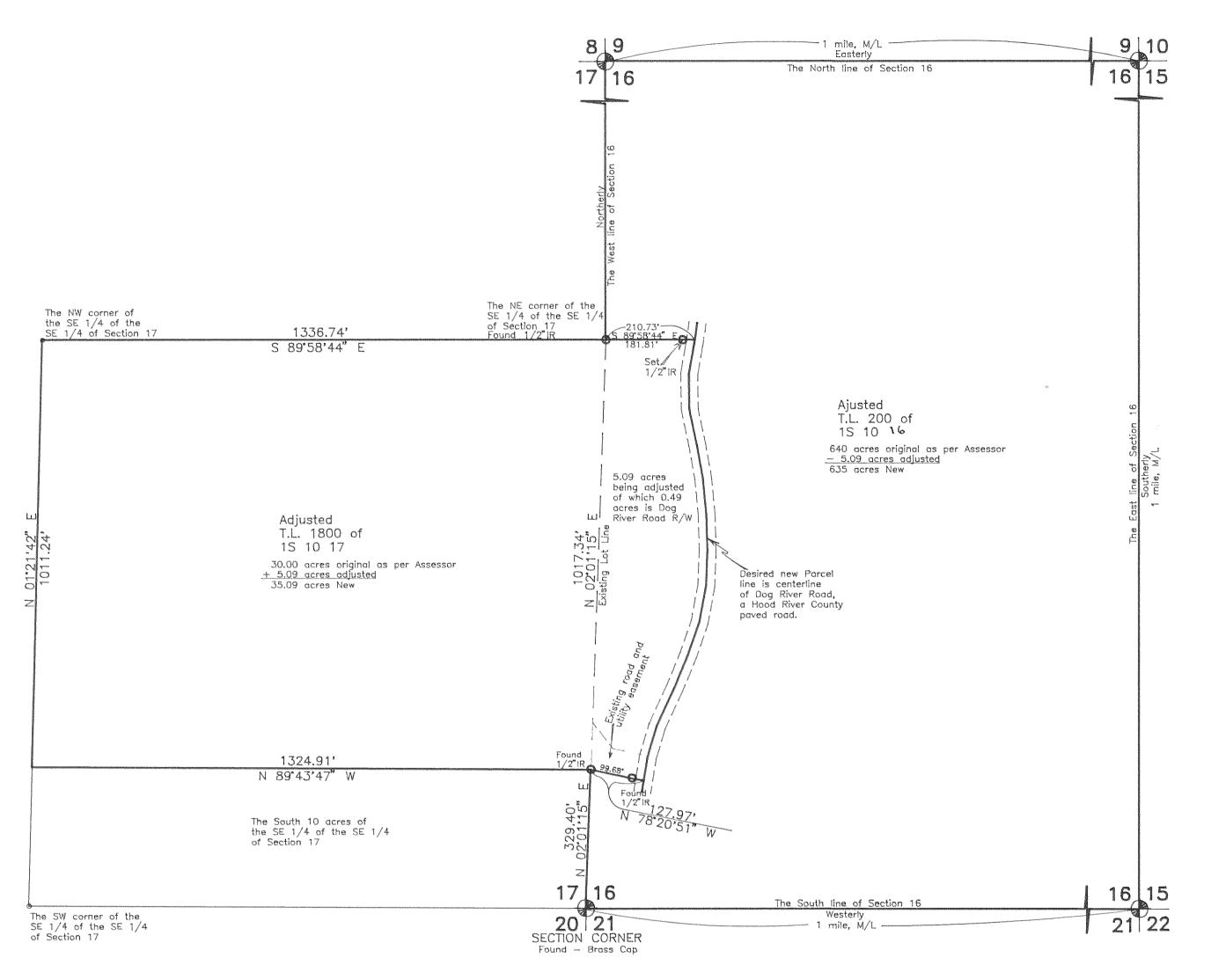
Basis of bearing and survey control as per D.L.C. C.S. 86012.
