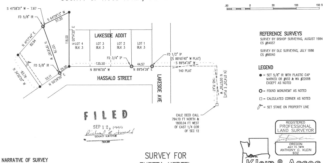
THE PURPOSE OF THE SURVEY WAS TO LOCATE THE CORNERS OF THE HEREIN SHOWN PARCEL. ALL MONUMENTS FOUND AND ESTABLISHED ALONG WITH THE MEASURED BEARINGS AND DISTANCES ARE SHOWN HEREIN.
