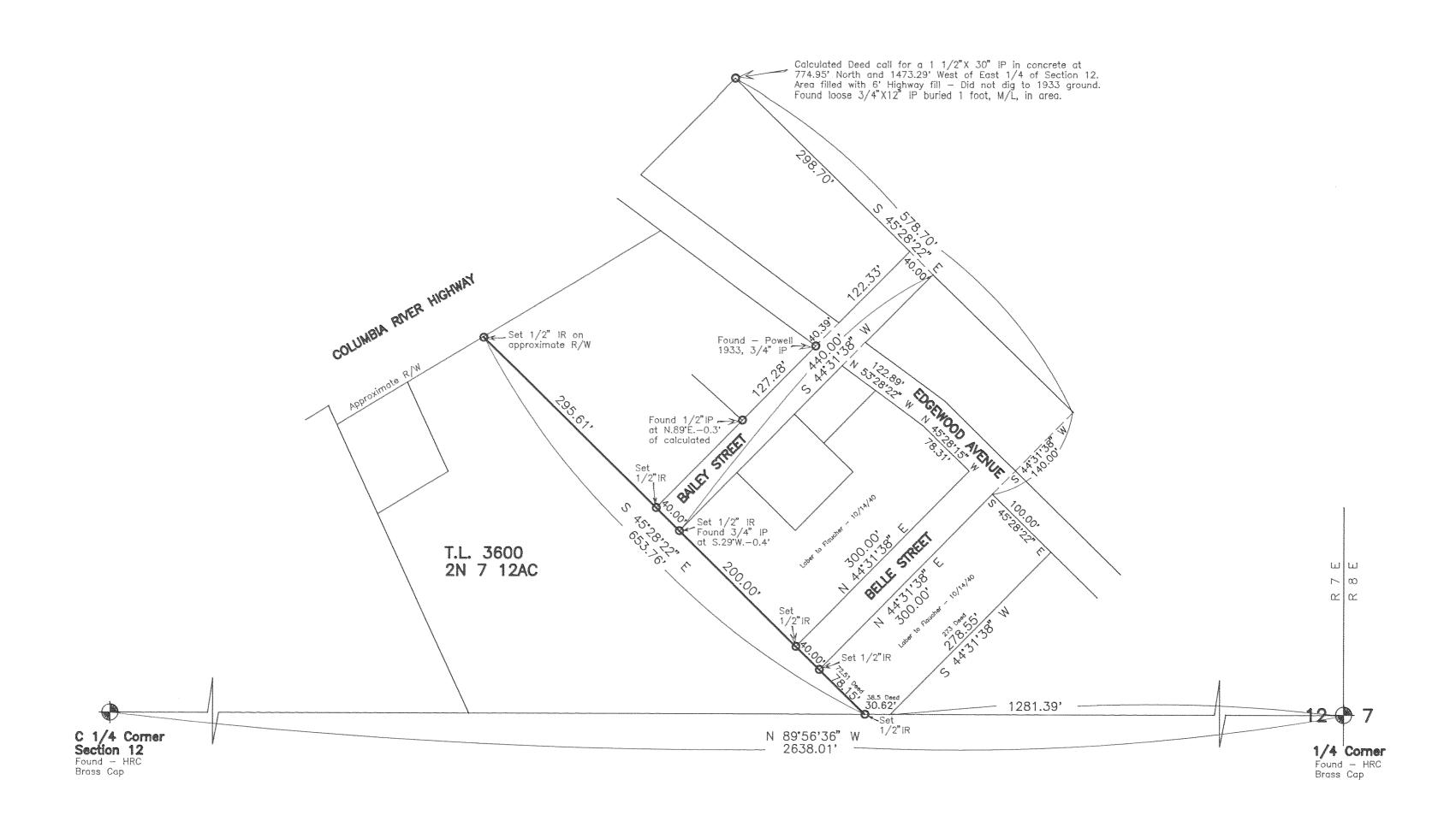
Basis of Bearing as per Deeds rotated 00°02'18" clockwise
